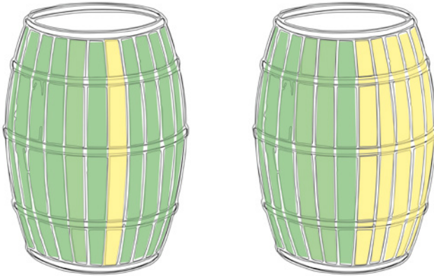
FIGURE 5 Casks made of timber from multiple provenance areas. (Left) A cask with timber from several provenance areas, where at least one stave is from a different provenance area than the rest. (Right) A cask with multiple staves from different provenance areas. The yellow and green colors indicate timber from different provenance areas.
