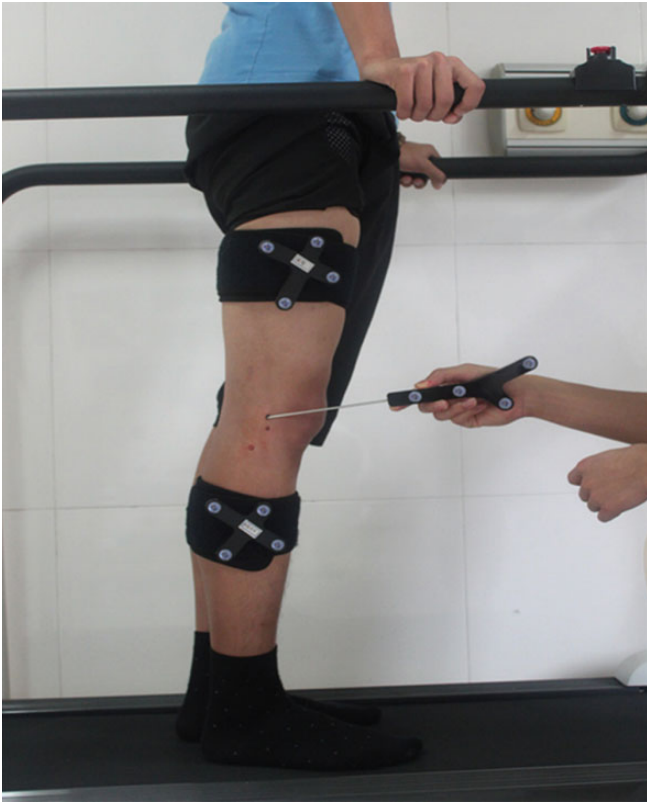
Figure 2. Two rigid bodies, each fitted with 4 infrared light-reflecting markers (OK_Marquer), were fixed to the participants' thighs and lower legs using bandages. A handheld digitizing probe with 4 infrared light-reflecting markers was used to determine the femoral and tibial anatomic landmarks.
