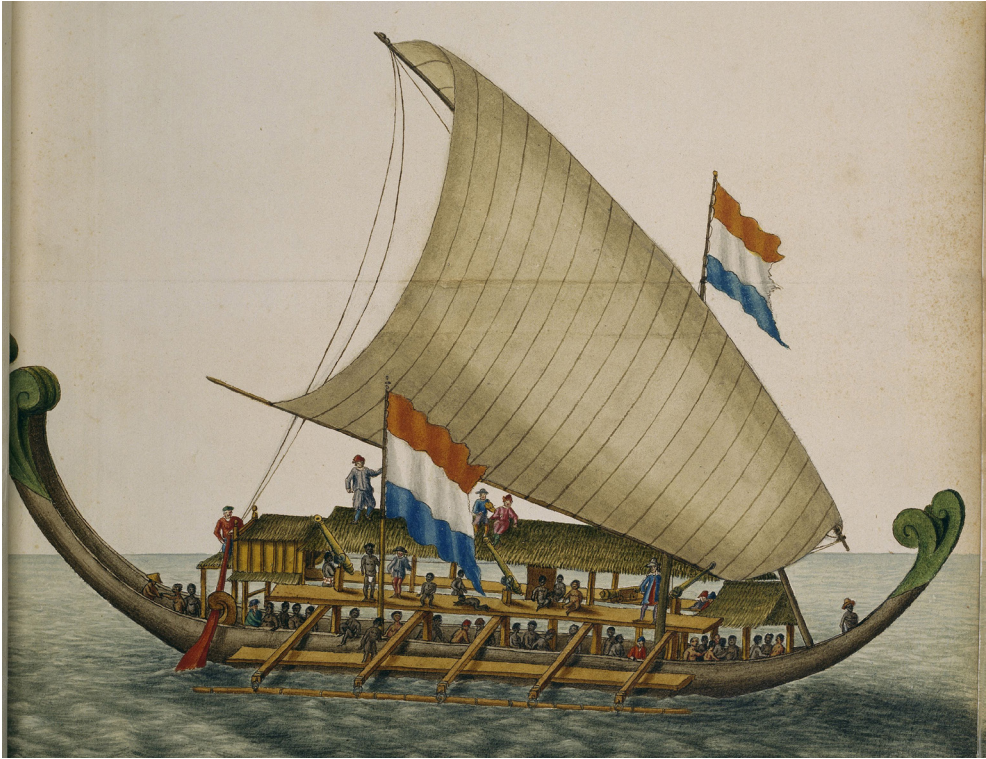
Fig 4.4 A kora-kora as depicted by Johannes Vingboons in the Atlas Blaeu – Van der Hem (c. 1665). The outrigger is a particularly distinctive feature of the kora-kora. Larger examples of these vessels, such as that depicted here, had sails and an elevated platform. Atlas Blaeu-Van der Hem, collection Austrian National Library, Van der Hem 40:16.
