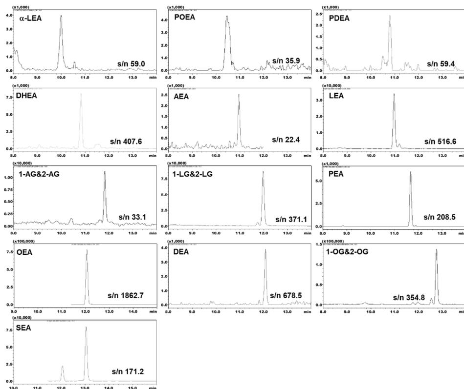
**Figure 5.** SRM chromatograms of eCBs and eCB analogues in pooled human CSF as determined by micro-LC-MS/MS using a flow rate of  $4 \mu\text{L min}^{-1}$  and an injection volume of  $3 \mu\text{L}$ . The x-axis is retention time and the y-axis is the detector response signal.
