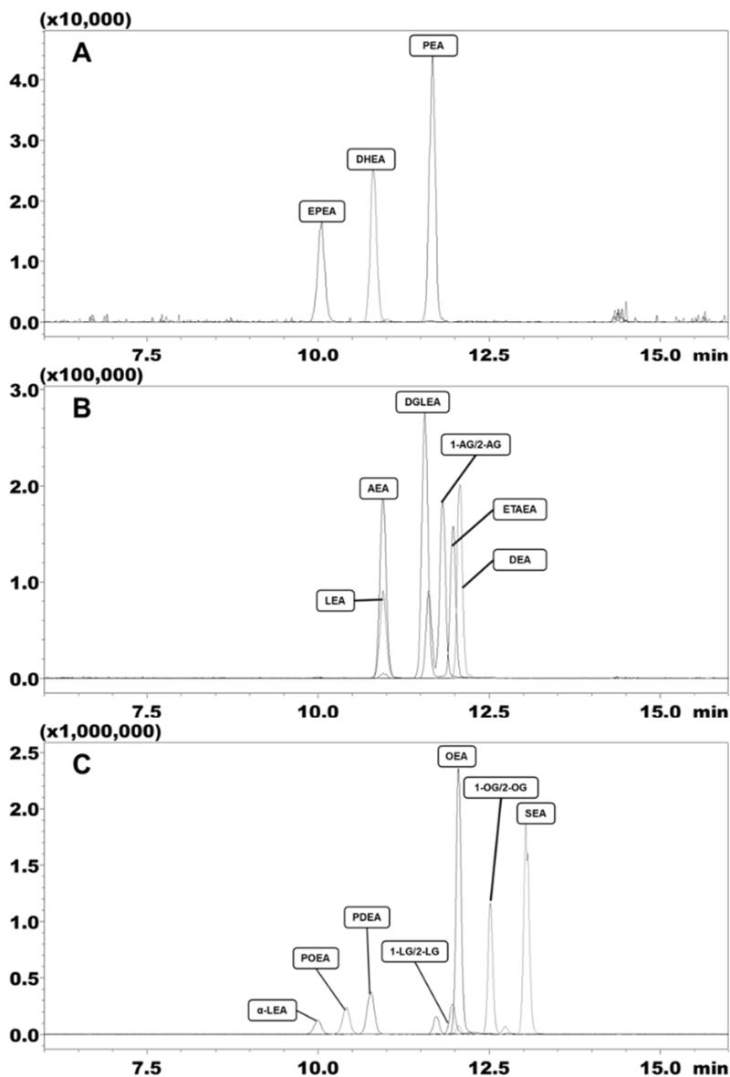
**Figure 4.** Overlay of SRM chromatograms of eCBs and eCB analogues obtained with the injection of standard solution II. The three panels represent the same chromatogram in different scales. (A) compounds with  $1 \times 10^4$  scale intensity (B) compounds with  $1 \times 10^5$  intensity scale (C) compounds with  $1 \times 10^6$  intensity scale.
