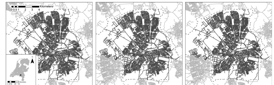
Figure A1.1, natural gas infrastructure in Eindhoven in 2020 (left), the situation in 2050 with 45% of buildings still connected to the gas grid (middle) and the situation in 2050 with 20% of buildings connected to the gas grid (right):
