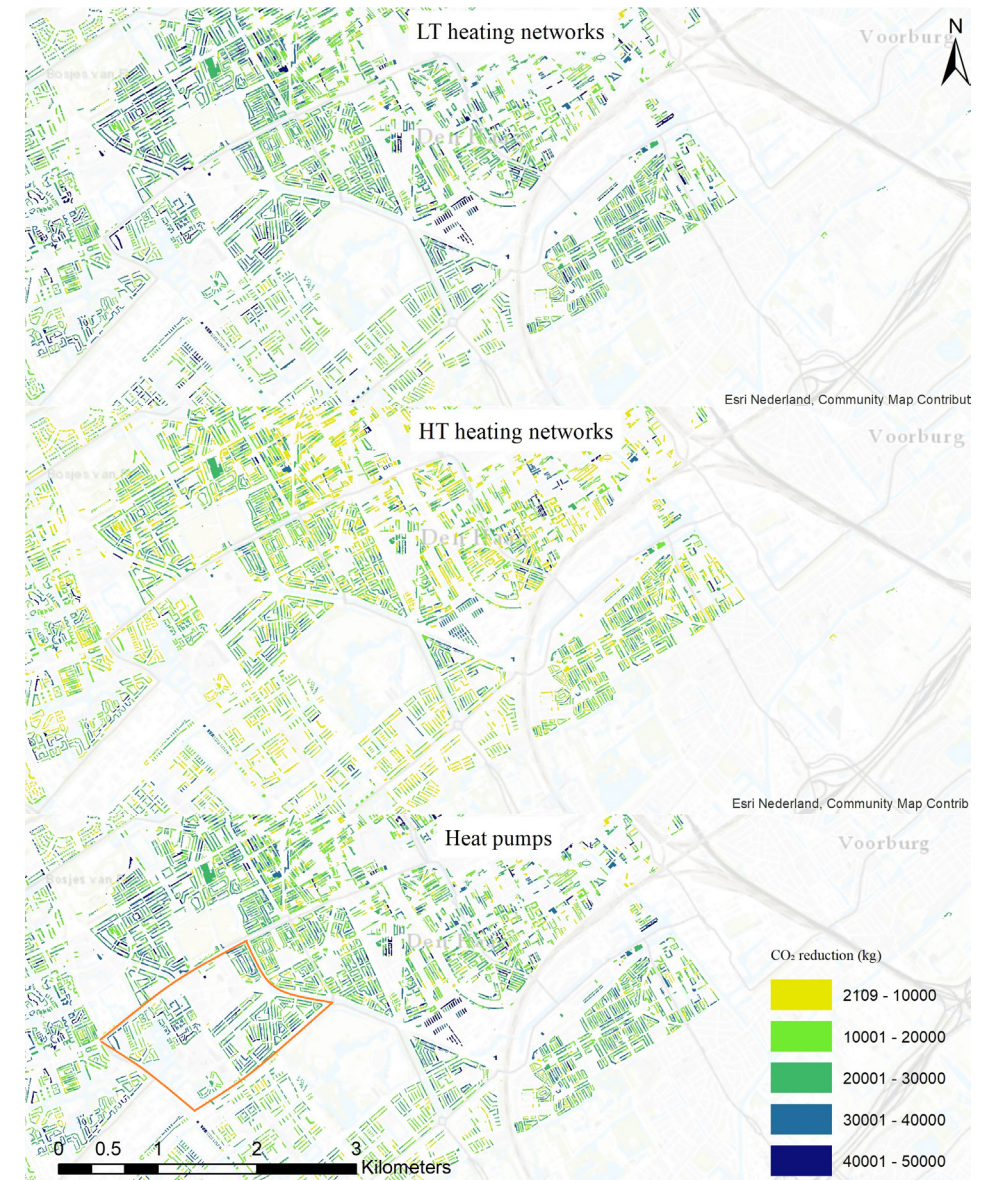
Figure 7, Annual CO 2 reduction potential for the alternative heating technologies per ZIP code in the city of The Hague (city districts best suited for a certain technology highlighted in orange): (a) LT heating networks; (b) HT heating networks; (c) Heat pumps.
