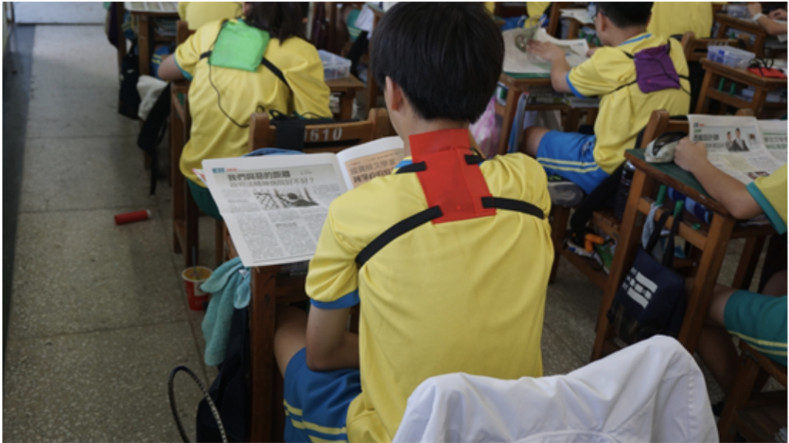
Picture 2. Three eighth graders wear Micro:bit enhanced devices to monitor sitting postures.
