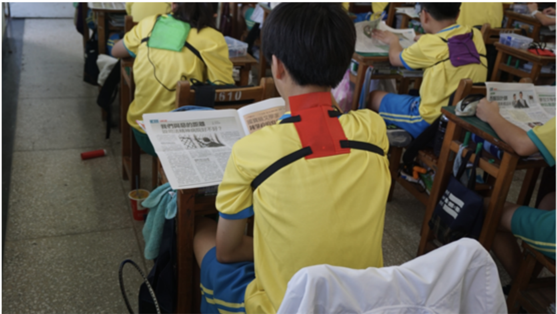
Picture 2. Three eighth graders wear Micro:bit enhanced devices to monitor sitting postures.
