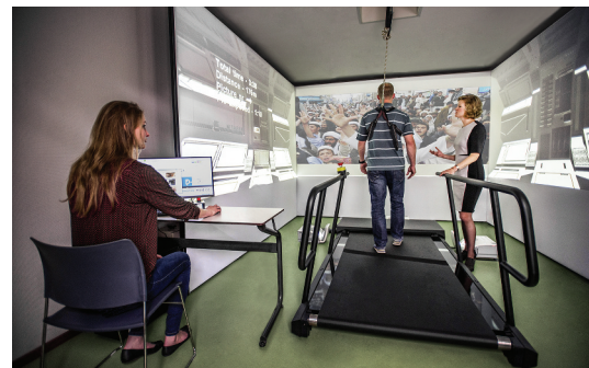
Figure 2. Image of the 3MDR set-up. The hardware included a dual-belt treadmill, a 180° projection on 3 screens by 3 projectors, and a surround sound system. The software consisted of a purpose-built virtual environment to walk in, personalized for each patient with images and music selected by patients. Participants wore a harness whilst on the treadmill for safety reasons. The therapist was standing alongside the veterans. A junior psychologist operated hardware and software.
