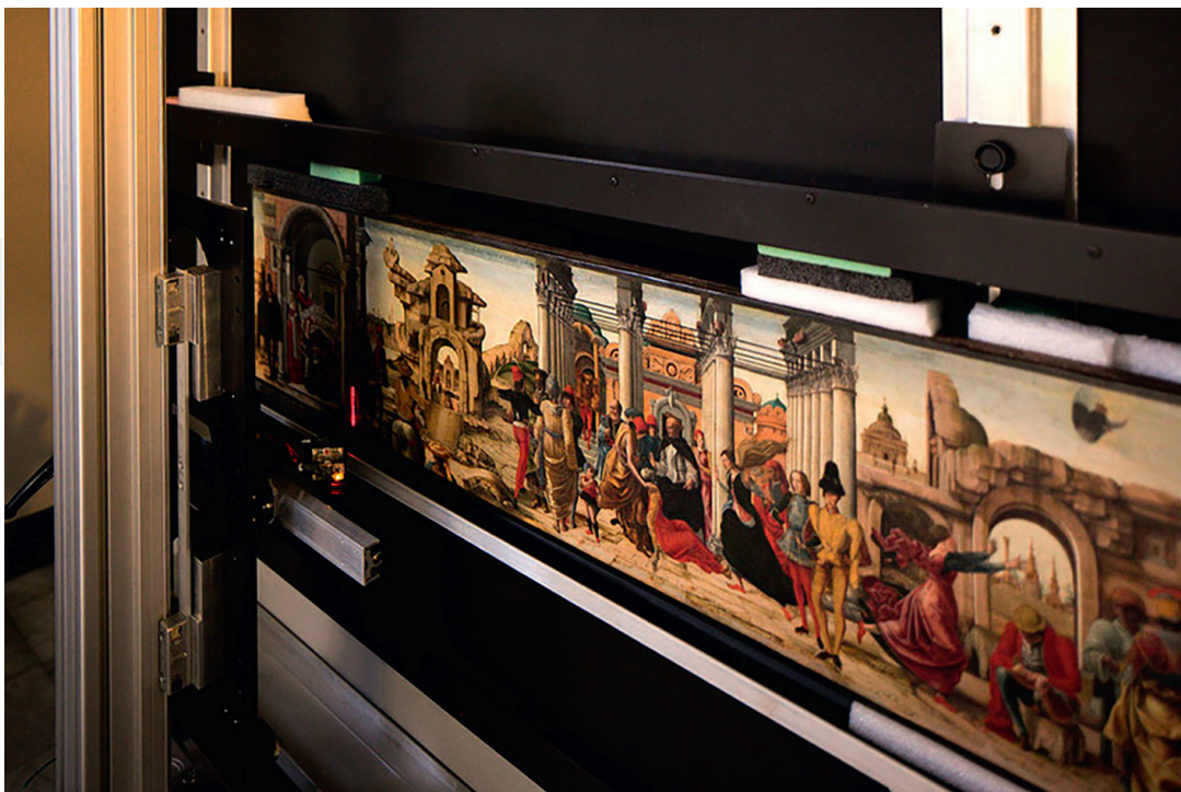
Figure 6. Recording the surface relief of Ercole De'Roberti's Stories of Saint Vincent Ferrer , predella of the Politico Griffoni, at the Pinacoteca Vaticana. Photo credits: Grégoire Dupond for Factum Foundation.
