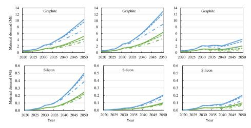
Supplementary Fig. 2.26: Primary battery material demand in the NCX (a), LFP (b) and Li-S/Air (c) scenarios from 2020 to 2050 without recycling, with recycling, and with recycling and second life. Here recycling refers to hydrometallurgical recycling as an example.
