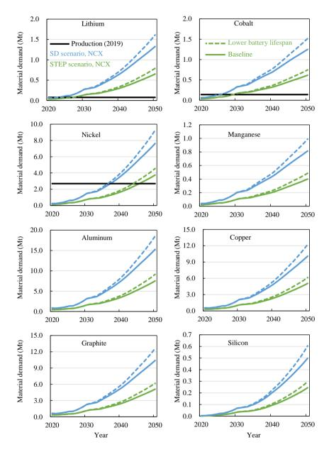
Supplementary Fig. 2.9: Result of sensitivity analysis of lower battery lifespan (*i.e.*, one EV will use 1.5 battery packs on average after 2020, while in the baseline scenario one EV will use 1 battery pack after 2020) on annual demand for Li, Co, Ni, Mn, Al, Cu, graphite, and Si in 2020-2050 without recycling.
