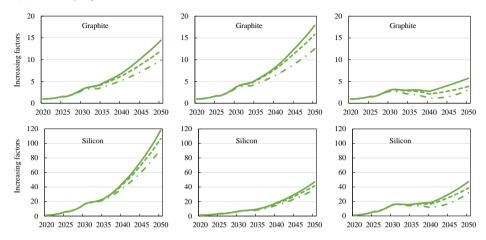
Supplementary Fig. 2.19: Increasing factors for the primary demand for Li, Ni, Co, Mn, Al, Cu, graphite, and Si from 2020 to 2050 in the STEP scenario in the NCX (a), LFP (b) and Li-S/Air (c) scenarios. Here recycling refers to hydrometallurgical recycling as an example.
