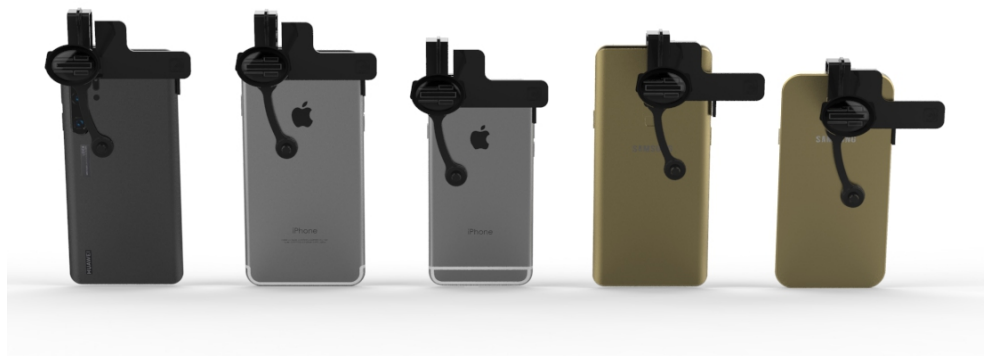
Figure 6.5: Render of iSPEX 2 attached to several smartphones with different dimensions and camera locations, seen from the back. Each has a backplate with unique positioner locations to place the optics directly in front of the camera.
