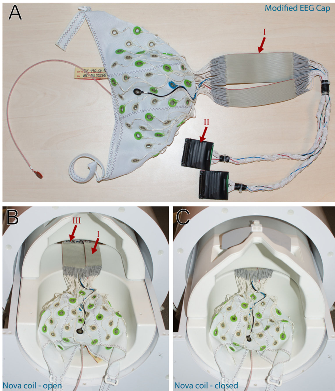
Fig. 1. The cable of the adapted 64 channel EEG cap is designed to fit the NOVA head coil. Indicated by the arrows are the adapted flattened cable (A) and connectors (B) and the small gap between the two halves of the NOVA coil through which the flattened cable is led (C).
