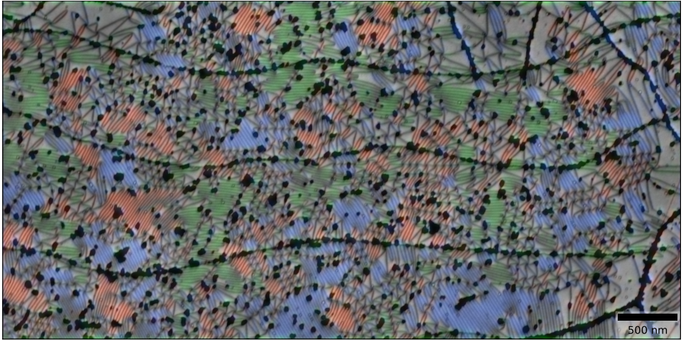
Figure 7.10: Area in Sample A with the GPA amplitudes corresponding to the three directions of stripe domains overlaid in red, green and blue.
