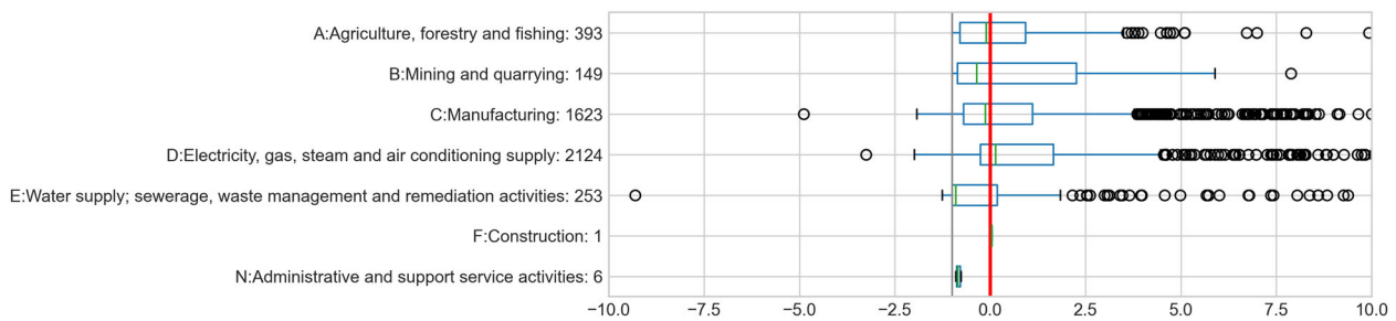
FIGURE 3 Relative deviation of the carbon footprints for all matched products across International Standard Industrial Classification (ISIC) section levels. The number in the y-labels indicates the number of matches (18 products from ecoinvent could not be included in this comparison due to the missing ISIC section level information). The red line is where ecoinvent and EXIOBASE CFs are equal. Numbers smaller than -1 (grey line) are negative CF results in EXIOBASE. Boxplots: The boxes represent the quartiles 2 and 3, where the green line is the median. The whiskers extend to 1.5 times the interquartile range and outliers are shown as circles. For readability, the plot has been cut-off at \pm 10 as certain outliers are several orders of magnitude higher/lower. The data behind this figure are provided in Supporting Information S2
