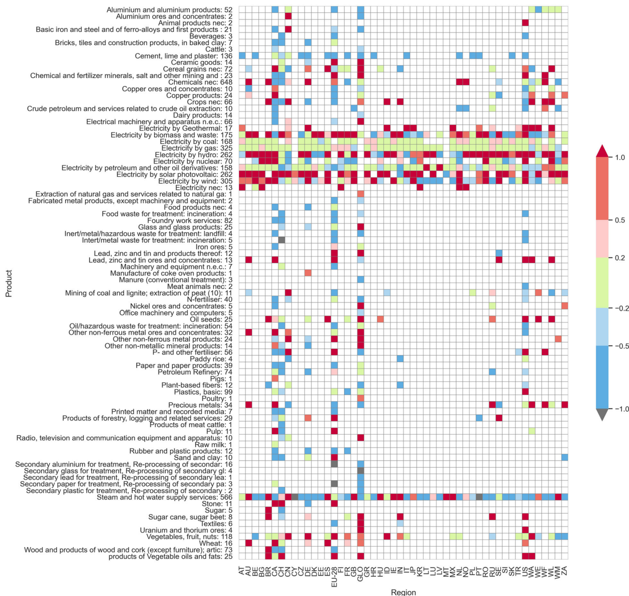
FIGURE 4 Median relative deviation of carbon footprints in ecoinvent from EXIOBASE by EXIOBASE product (y-axis) and regions (x-axis). The colors relate to the value of the relative deviation: Blue means that ecoinvent CFs are lower and red means that ecoinvent CFs are higher. RoW EXIOBASE regions are: Asia and Pacific (WA), RoW America (WL), RoW Europe (WE), RoW Africa (WF), and RoW Middle East (WM). The number in the y-labels indicates the number of matches. The data behind this figure are provided in Supporting Information S2
