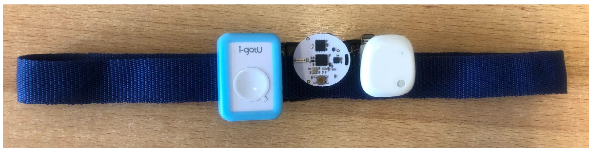
Figure 3. The proposed sensing system: GPS logger, proximity tag, MMR sensor (from left to right) mounted on a belt.
