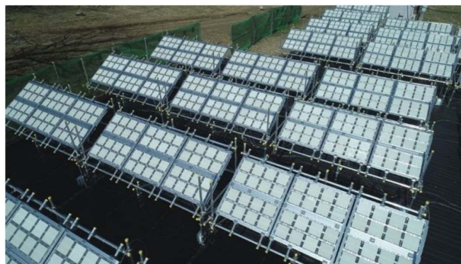
Figure 9. An example of field test of solar hydrogen production by photocatalytic water splitting. Reprinted from [69] with permission. Copyright Agency for Natural Resources and Energy.
