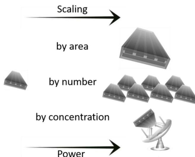
**Figure 11.** Possible scaling strategies of a photoelectrochemical device: (i) scaling by size, which includes the increase in the photoabsorber area, (ii) scaling by number, which includes the multiplication and connection of sizable units, and (iii) scaling by concentration, which includes the increase in irradiation concentration. All approaches (which can also be combined) will increase the input and output power of the system.
