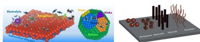
**Figure 31.** Illustration of catalyst surface effects on the CO<sub>2</sub>RR activity and selectivity. Reproduced with permission from [178, 179].
