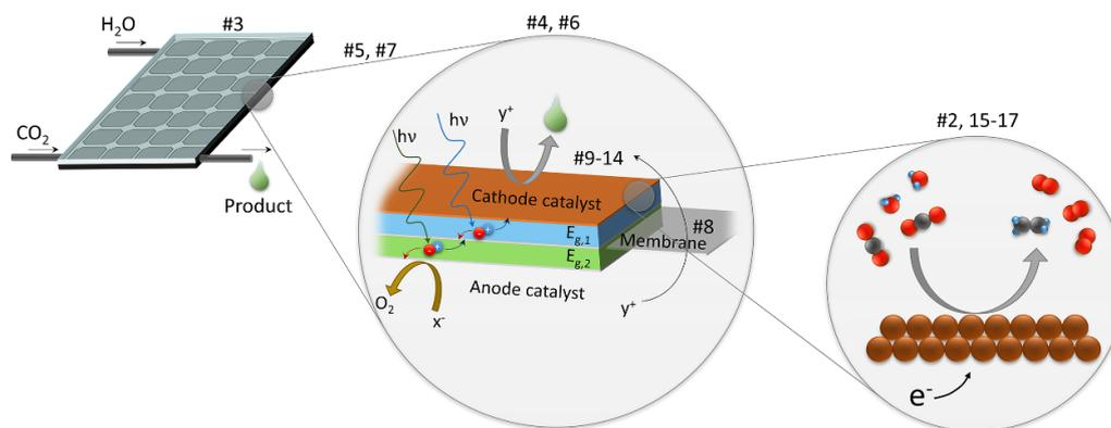
**Figure 1.** Conceptual drawing of a solar fuel generator (left), showing the functional layers of the device (middle) and the atomic-scale electrochemical processes that occur at the catalytically active surfaces. The numbers indicate the section addressing every component or challenge.
