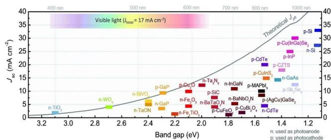
**Figure 20.** The state-of-the-art photocurrent density ( $J_{sc}$ ) of photoelectrodes for PEC water splitting under standard conditions of 1.0 sun at 1.23  $V_{RHE}$  for photoanodes and 0.0  $V_{RHE}$  for photocathodes. Adapted from [31] with permission from the Royal Society of Chemistry, copyright 2019.
