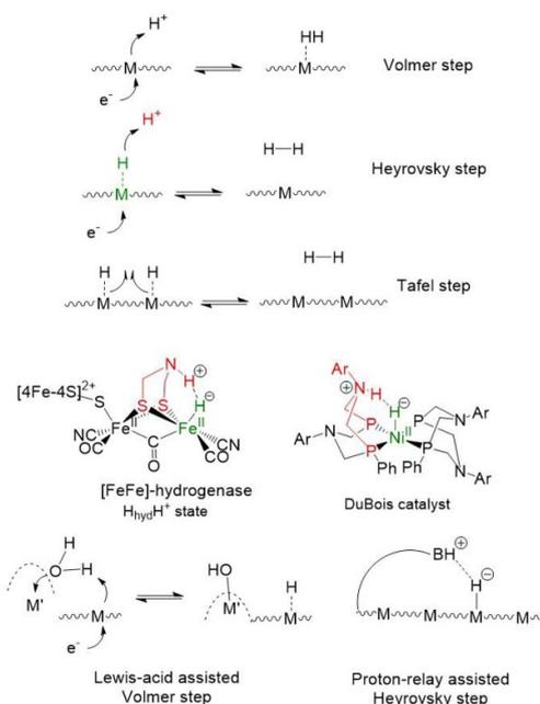
**Figure 28.** Key steps involved in the HER (top), involvement of proton relays at the active site of [FeFe]-hydrogenases and bioinspired DuBois' catalyst (middle) and possible implementation of such molecular mechanisms at inorganic surfaces (bottom).
