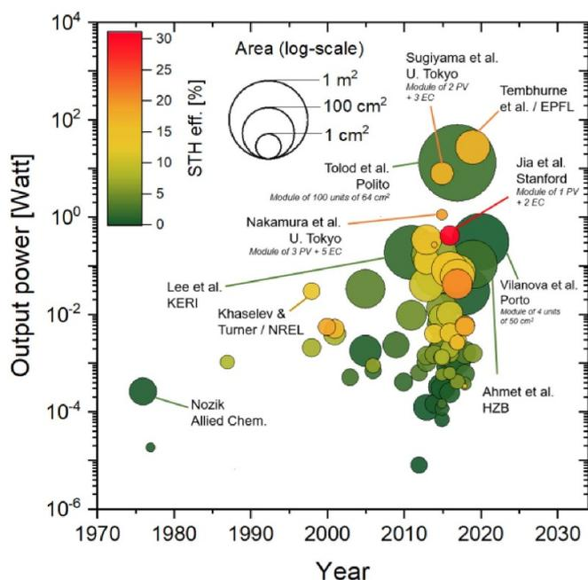
**Figure 12.** A comparison of photoelectrochemical water splitting devices (i.e.  $\text{H}_2$  production) reported in the literature, taken from the combined lists of [35, 81]. The reported solar-to-hydrogen (STH) efficiency, device active (i.e. light absorber) area and the corresponding output power of the devices are shown. Five modular devices where multiple units are combined (i.e. scaling by number) are also identified.
