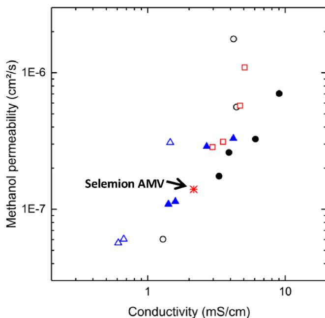
**Figure 13.** Experimental tradeoff between electrolyte ionic conductivity and CO<sub>2</sub> reduction product (methanol) permeability for a series of poly(vinyl imidazolium) membranes. For reference, a commercial anion exchange membrane, Selemon AMV, is indicated. Reproduced from [85] with permission from the Royal Society of Chemistry.
