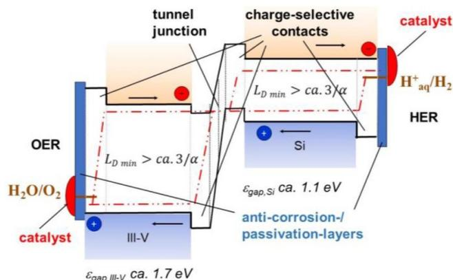
**Figure 15.** An idealized electronic band diagram and the charge carrier trajectories in a Si/III–V tandem structure plus surrounding functional layers, catalysts, Fermi-levels, and redox potentials for water splitting.
