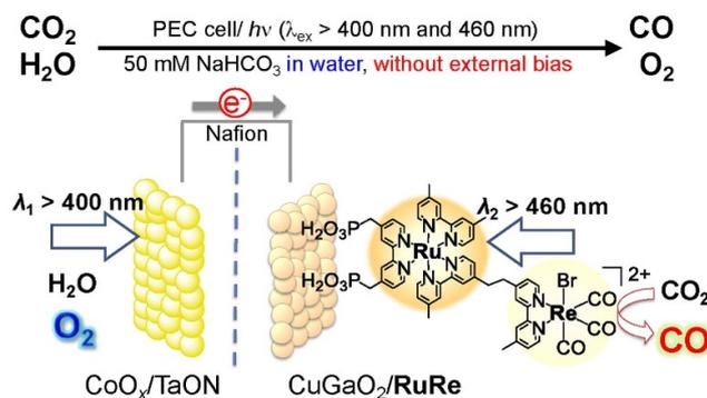
**Figure 23.** Photocatalytic hybrid systems of the Ru(II)-Re(I) supramolecular photocatalyst for CO<sub>2</sub> reduction with (a) periodic mesoporous organosilica as light harvester and (b) semiconductor photoelectrodes for water oxidation.
