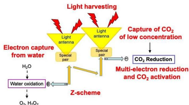
**Figure 22.** Required functions for CO<sub>2</sub>-reduction photocatalytic systems.
