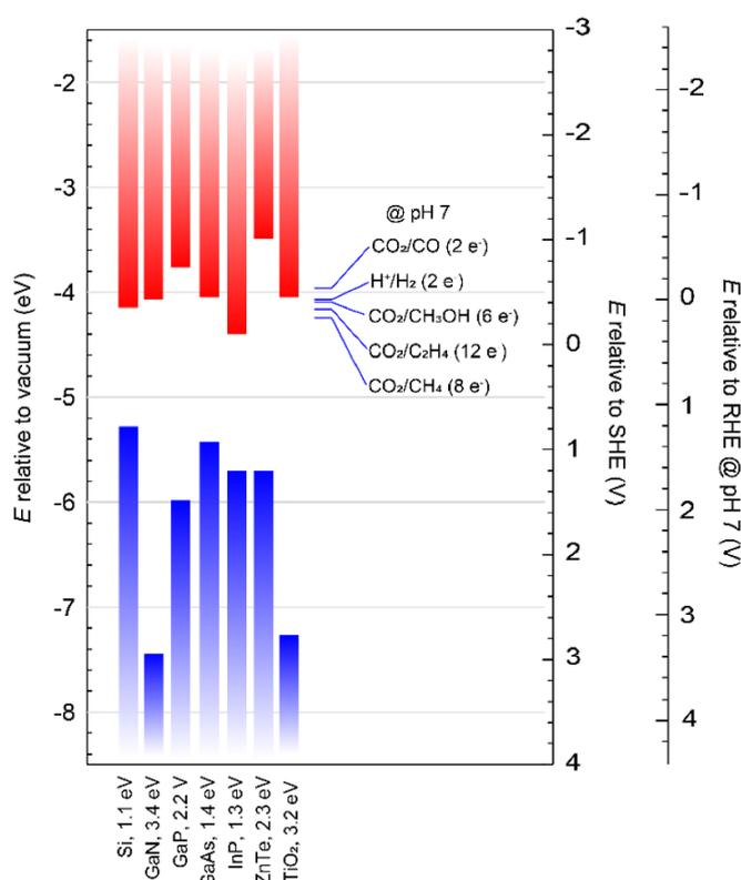
**Figure 24.** Schematic band alignment for selected group IV, III-V, II-VI, and oxide semiconductors with the valence band shaded in blue and the conduction band in red. The equilibrium potentials for CO<sub>2</sub> reduction reactions and for the hydrogen evolution reactions are also shown for pH 7, a typical experimental condition.
