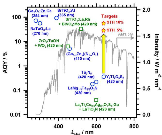
**Figure 10.** Relationship between the absorption edge wavelength ( $\lambda_{\text{abs}}$ ) and the apparent quantum yield (AQY) for overall water splitting of some photocatalysts. Circles and squares represent one-step and two-step excitation systems, respectively. The wavelengths at which the AQY values were measured are shown in parentheses. The power spectrum of the reference sunlight (air mass 1.5 G) is also plotted on the right axis for comparison.
