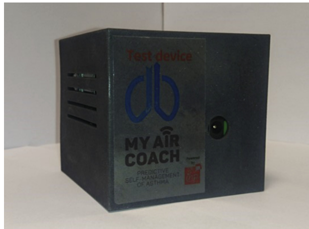
FIGURE E2. myAirCoach air quality monitor. The indoor air quality monitor is capable of measuring several indoor parameters such as nitrogen dioxide (NO 2 ), sulfur dioxide (SO 2 ), particulate matter (PM2.5 and PM10), humidity, air pressure, and temperature.
