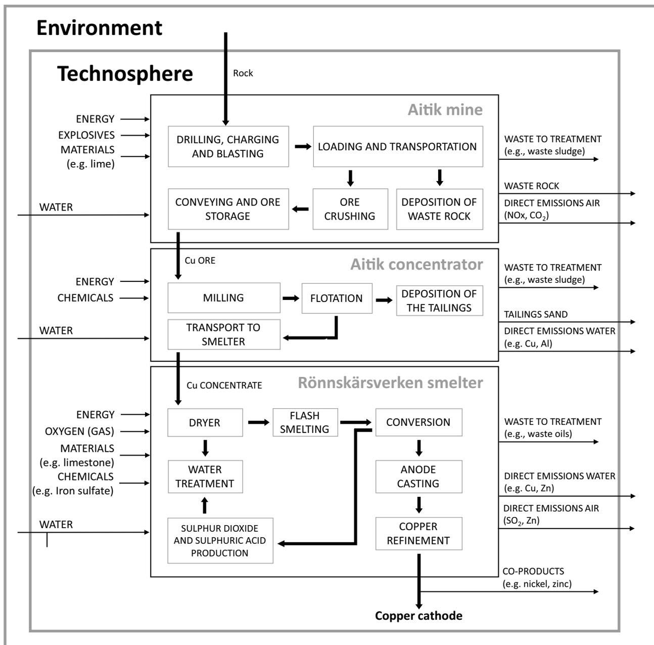
**Fig. 1** Flow diagram of the copper production system showing the Aitik operation, including the Rönnskär smelter. Only primary processes that are relevant for copper are shown. Boxes represent processes, thick arrows represent copper flows and flows within the sys-
