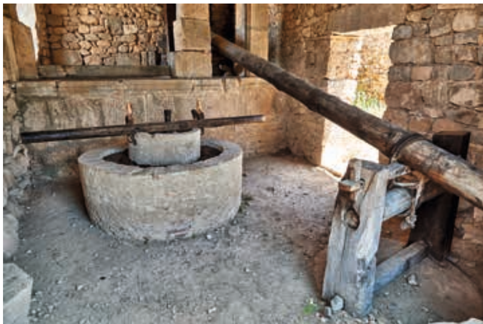
FIGURE 3.6 Reconstructed installation for pressing olives in a house at Volubilis, Roman province of Mauretania Tingitana (Morocco). Photo: Juergen Ritterback / Getty Images.
