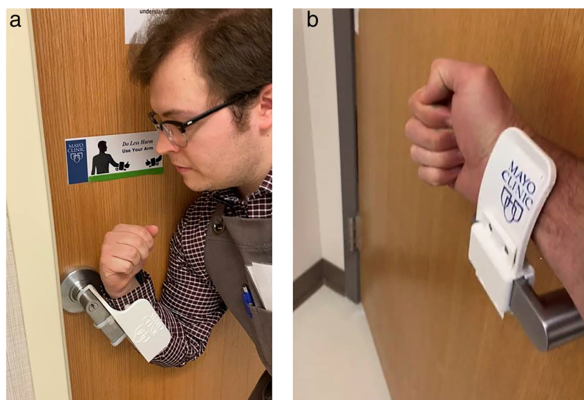
FIGURE 4: Three-dimensional-printed plastic door handle paddles to enable easy opening of doors with an elbow or forearm, reducing hand contact with the door latch. Different designs allow for opening while (a) pushing the door open or (b) pulling the door open. Images courtesy Dr Jonathan Morris, Mayo Clinic, Anatomic Modeling Unit, Rochester, MN.
