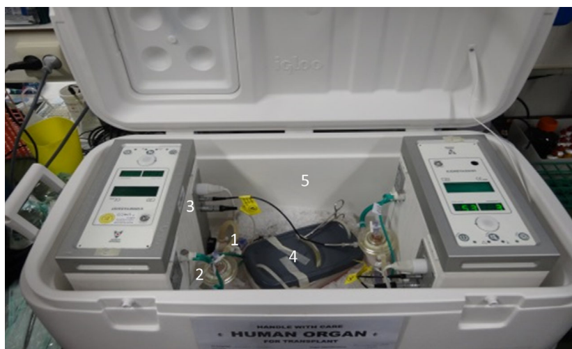
Figure 1 Transportable dual arterial oxygenated hypothermic machine perfusion device. The perfusion system consists of two separate centrifugal pumps (1), two hollow fiber oxygenators (2), perfusion pressure, flow and temperature sensors (3), an organ holder (4) in an insulated container filled with melting ice (5).
