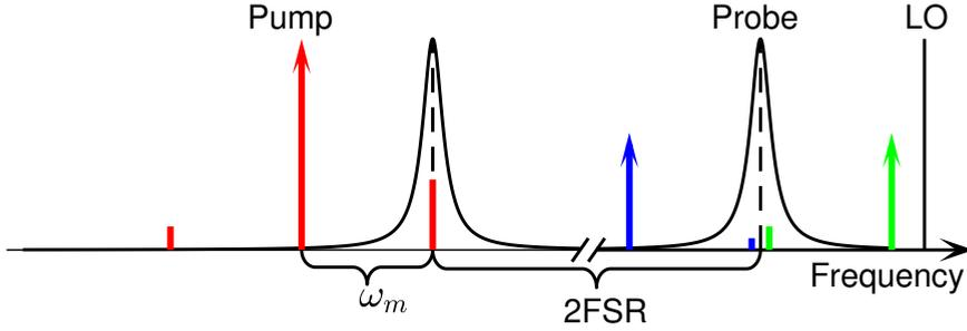
**Figure 7.2:** Sideband cooling experiment with two off-resonant probes. The probes are detuned by  $\Delta = \pm(\omega_m + \delta)$  such that the Stokes and anti-Stokes sidebands are separated by more than  $\Gamma_{\text{opt}}$  to avoid interference between them.  $\Gamma_{\text{opt}} \ll \delta \ll \kappa$ .
