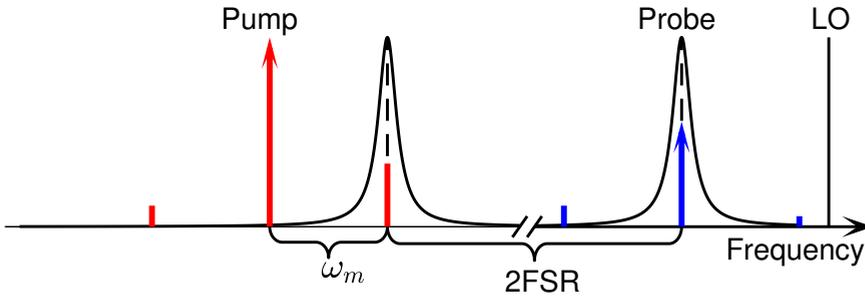
**Figure 7.1:** Sideband cooling experiment with resonant probe. The Stokes and Anti-Stokes sidebands from the resonant probe are detected via heterodyning with local oscillator (LO), the ratio of the sidebands provides information of the thermal state of the mechanical mode.
