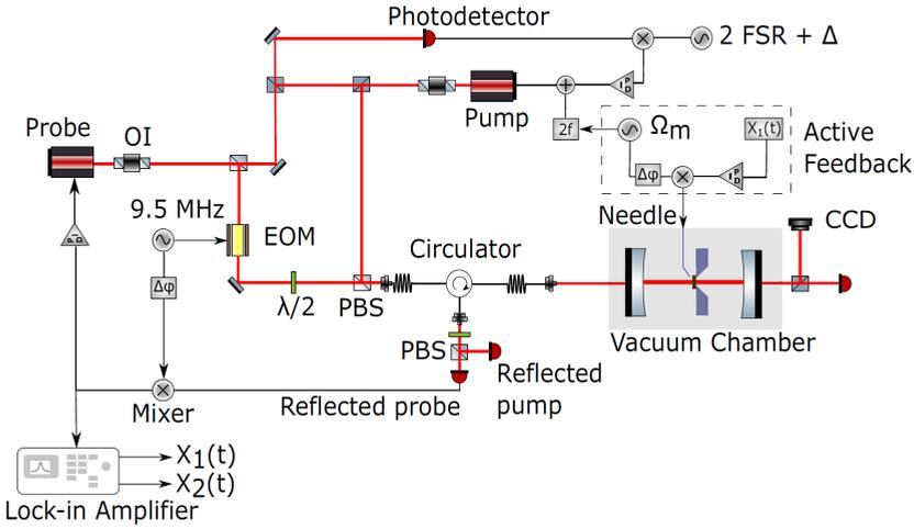
Figure 2.3: Optical setup.
