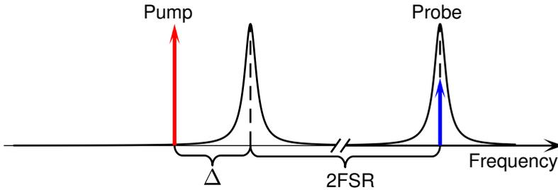
Figure 2.4: The probe and pump laser frequencies.
