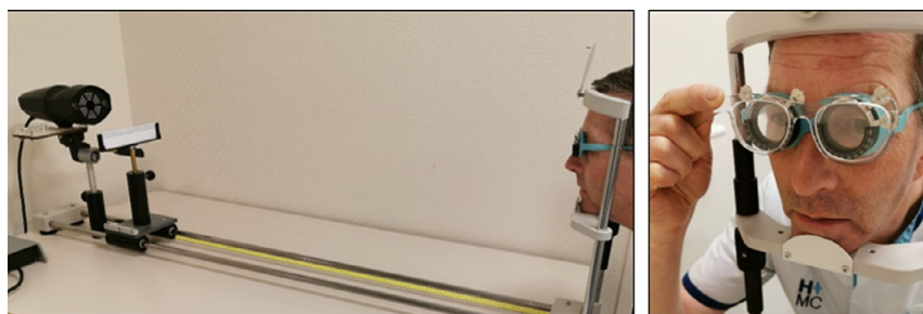
Fig. 1. Test set-up using an adult subject; positioned at 1-metre distance from the Plusoptix PowerRefractor, wearing a trial frame with full Retinomax refractive values. A Radner LogMAR reading chart text representing 0.8 decimal was attached directly under the measuring device. Subjects read the text loudly, while the text was slowly moved towards the subject. In case of failure due to a large pupil size, a 0.04 ND filter was used to attenuate the transmitted infrared light. [Colour figure can be viewed at wileyonlinelibrary.com ]
