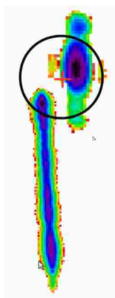
Figure 2.13: Illustration of the algorithm that leads to the construction of the on model centroid image for a stack. Shown are two of the reflected beam images. The cross at the center indicates the place where the barycenters of the reflected beams are expected to fall if the sample behaved ideally. A synthetic image, called the on model centroid image, is obtained by adding each reflected beam to it after applying the translation calculated during the analysis.
