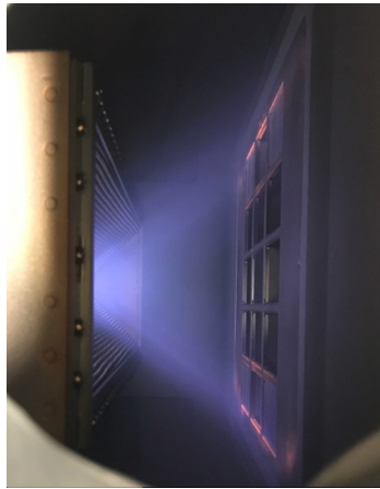
Figure 3.1: Views of the coating chamber from above. (a) Schematic view displaying the position of the inverse sputter etcher (ISE) compared to the Iridium target and its magnetron. The carriers holding the substrates are mounted on a rotating ring passing by the ISE and the Iridium target successively. Note that two additional magnetrons are available in the chamber and that a door is used to load and unload the carriers. (b) Discharge plasma glow of the ISE. The ISE is visible on the left of the picture and the carriers with the substrates on the right.
