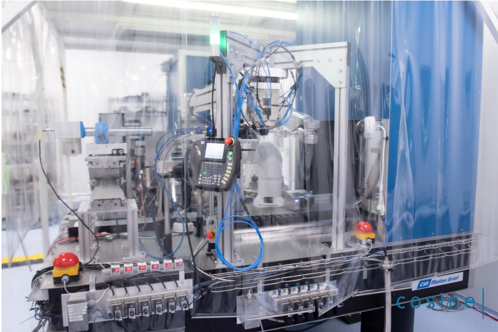
Figure 2.7: Stacking robot inside a cleanroom, as installed at cosine. It is equipped with a robotic arm to extract plates for stacking. A hexapod allows aligning the mandrel to the die. The blue box on the right is an optical metrology system that can measure the figure and cleanliness of each plate after having been stacked.
