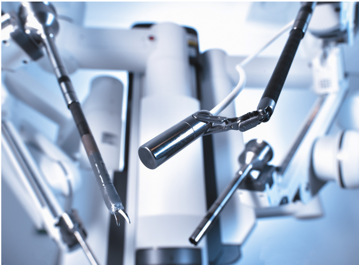
Fig. 1 – Zoomed-in photograph of the prototype DROP-IN gamma probe as grasped by a ProGrasp instrument of the da Vinci surgical robot. Copyright H.J.F. van de Stadt (used with permission).
