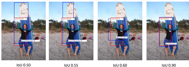
Figure 3.4: IoU example: The red color box and blue color box come from MS COCO and Visual Genome, respectively, and the IoU value of two different boxes of the same object should be high.
