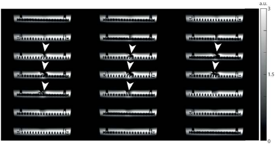
Supporting Information Figure 1. A) Titanium aneurysm clip (2 cm), used in the phantom and in-vivo scans, placed on the phantom; a plastic grid with 8.0 mm periodicity. B) Reformat demonstrating the distortion of the slice profile, indicated by white arrowheads, of the phantom as shown in A). Images were to demonstrate the through-plane effect.
