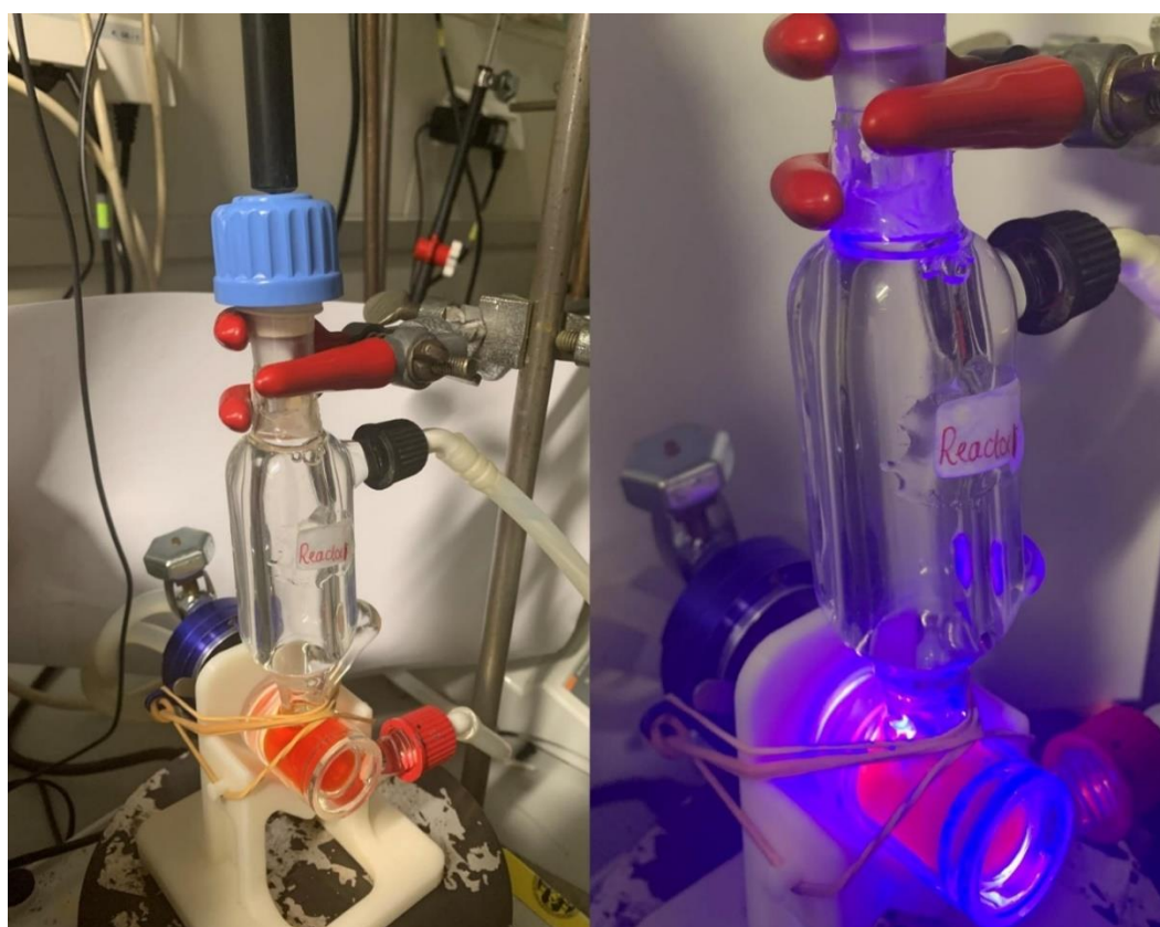
Figure AI.29 The photocatalytic set-up.
