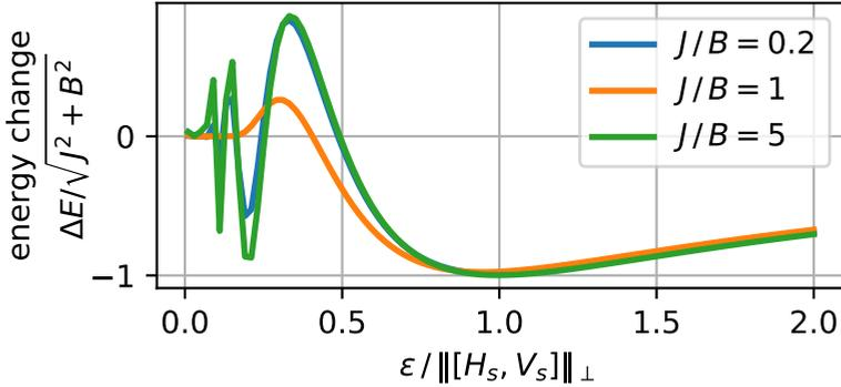
**Figure 6.5:** Change in energy expectation value for the application of a single cooling step to the maximally mixed state of a  $N = 8$  qubit transverse field Ising chain Eq. (6.4.5), depending on the fridge energy  $\epsilon$ . The coupling potential is  $V_S = Y_3$ , the Pauli  $Y$  on the third qubit. The relation  $B^2 + J^2 = 1$  fixes the energy scale.
