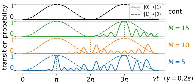
**Figure 6.2:** Effects of Trotterization on cooling and reheating probabilities as a function of the coupling time  $t$ , for different numbers of Trotter steps  $M$  per cooling cycle. Vertical dotted lines indicate the  $M$ -th reheating oscillation, at which point the Trotter approximation fails.
