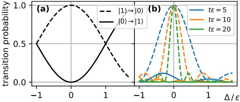
**Figure 6.3:** Effect of fridge-system detuning  $\delta = \Delta - \epsilon$  on the cooling (dashed lines) and reheating (solid lines) probabilities for **(a)** the bang-bang cooling approach, and **(b)** the weak-coupling cooling approach, where colors indicate different coupling strengths.
