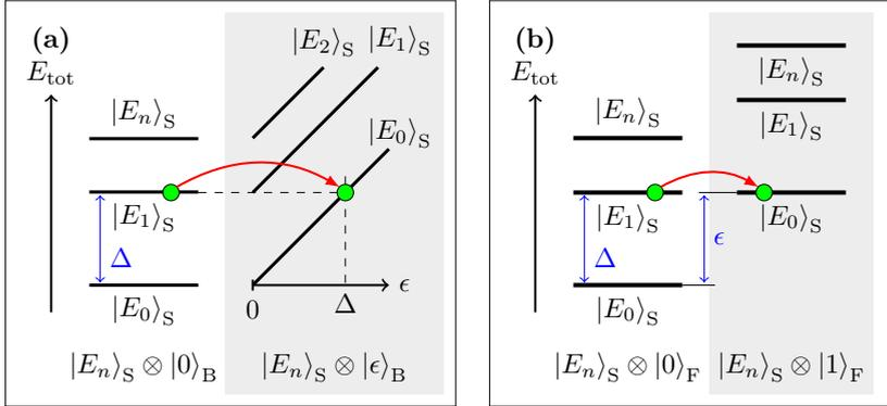
**Figure 6.1:** The de-excitation of the system transition  $|E_1\rangle_S \rightarrow |E_0\rangle_S$  mediated by: (a) a continuous-spectrum natural bath B, where an excitation  $|\epsilon\rangle_B$  at energy  $\epsilon$  is produced, and (b) a single-qubit digital fridge F, which can be excited if  $\epsilon = \Delta$ .
