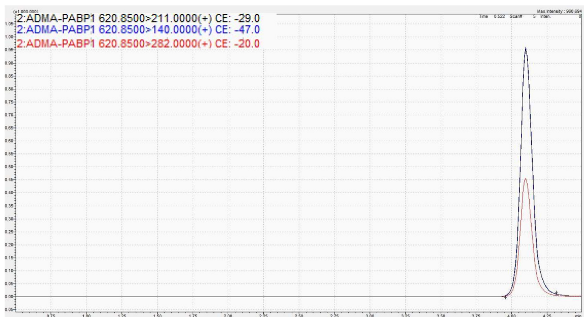
Figure S2. LC-MS/MS traces of PABP1 456-466 R 460 -aDMA (methylated product). MS method: 0.5-4.5 min; retention time 4.101 min, Q1 mass detection; 620.85; Q3 mass detection: 282.00, 211.00, 140.00.
