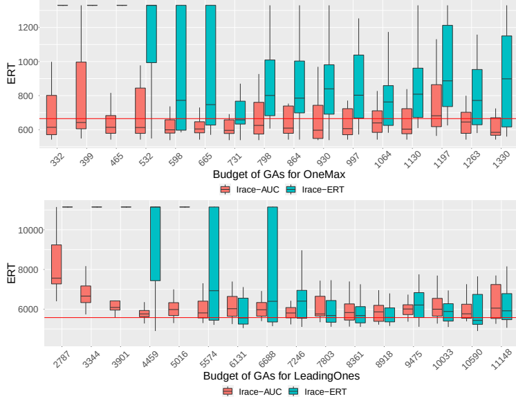
Figure 6.9: ERT values ( y -axis) of the GAs obtained by Irace for ONEMAX and LEADINGONES in dimension n = 100 , for different budgets B that the GAs can spend to find the optimum ( x -axis). Showing results for B \in \{(0.5 + 0.1t) \text{ERT}_{(1+1) \text{ EA}} \mid t \in [15]\} . For comparison, the ERT values of the (1 + 1) EA are plotted by horizontal red lines. Results are for the best found configurations obtained from 20 independent runs of Irace, and each of the ERT values is with respect to 100 independent validation runs.
