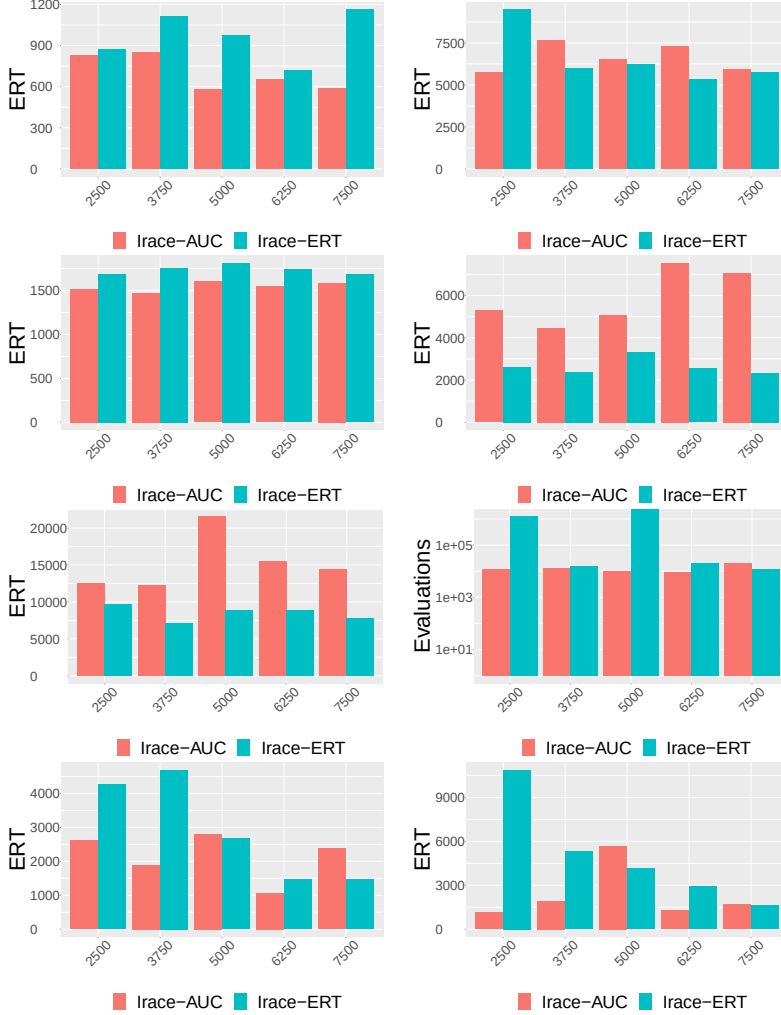
Figure 6.10: ERT values ( y -axis) of the GAs obtained by Irace with different configuration budgets B_T (the number of configurations that Irace can test, x -axis). Results are for B_T \in \{(0.5 + 0.25t)5,000 \mid t \in [4]\} . Each ERT value is for the 100 validation runs of the configuration suggested by Irace after a single run, i.e., one for each budget.
