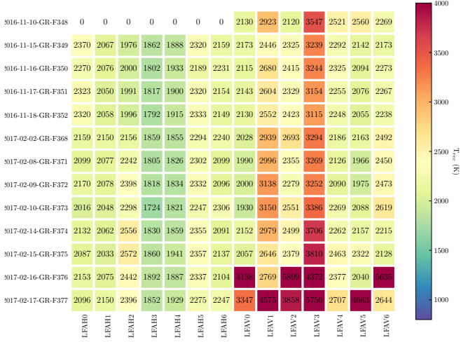
Fig. A.6: Summary of upGREAT LFA single sideband receiver temperature over the 13 project flights. Note the increase in receiver temperature for the V array towards later flights that was linked to a degradation in LFAV LO performance. The LO was shipped back to the manufacturer for maintenance after the flight series. The H LO was not available during the 2016-11-10 flight and is recorded here with 0 receiver temperature.
