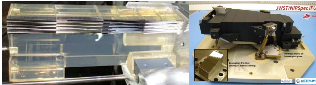
Fig 16: Left: The Image Dissector Array (IDA) manufacturing constitutes a WINLIGHT Optics/CNRS patent. Innovative methods, developed conjointly by LAM (Laboratoire d'Astrophysique de Marseille, France) and WinLight Optics (Marseille, France), allow reaching high performances (accurate roughness, sharp edges, surface form, etc.) with standard glass manufactured components while saving costs and time by an order of magnitude compared with classical techniques. This IDA is constituted by 48 slices. Right: Main picture: The NIRSpec IFU flight model. The IFU is roughly the size of a shoe box and weighs less than 1 kg. Insert: A diamond-machined image slicer, a key element of the IFU, pictured during manufacture. Credit: R. Sharples / University of Durham, United Kingdom.
