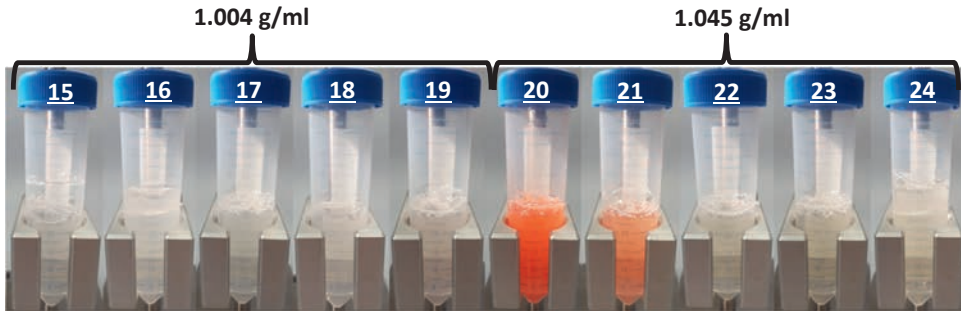
Figure S2. Centrifuge bowl outflow fractions. In order to simulate the crucial islet isolation step of changing medium from Ringer's acetate solution to University of Wisconsin solution (UWS), mock tissue was pumped into a continuous flow centrifuge bowl filled with Ringer's acetate solution (RAS). This was followed by an additional 250 ml Ringer's acetate solution (25 ml/min) and 250 ml UWS (25 ml/min). Fractions of 25 ml were collected via the overflow in 50 ml tubes. After 19 fractions of clear RAS, the 20 th fraction contained mock tissue with a density of 1.030 g/ml. Subsequent fractions all contained UWS with a density of 1.045 g/ml without other densities of mock tissue. The first 14 collected fractions are not shown. The continuous flow centrifuge bowl was set at 1500 RPM (145 g at the bottom of the bowl and 105 g at the top of the bowl). An increased centrifuge speed was chosen due to the higher viscosity of UWS to RAS (3.32 vs. \approx 1.56 mPa·s, respectively, at 4°C 41 ) and a higher density (1.045 vs \approx 1.004 g/ml, at 4 °C 53 ) of UWS to RAS. Also, since the density difference between the UWS and mock tissue is much smaller than in the retention and washing phase (when the tissue is in RAS), the sedimentation rate of the mock tissue is slower, requiring more time and therefore a lower pump speed.
