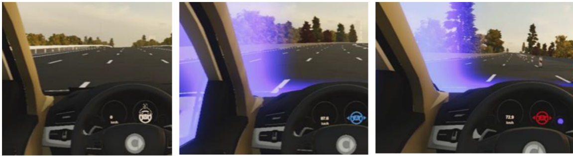
Figure 1: Left: the car in manual mode (icon on instrument cluster shows manual mode; started pulsing once AD mode was available); Middle: the car in automated mode (blue AD mode icon is displayed and the blue visual pattern in the windshield is active). Right: TOR (icon flashes red, and frequency of blue windshield visual pattern is rapidly increased).
