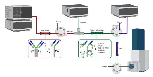
**Figure 1.** Schematic representation of the automated on-line bottom-up approach for mAbs using mD-LC-MS which enables on-line on-column reduction by RP-HPLC (1D), tryptic digestion (2D) and peptide mapping by RP-MS (3D).
