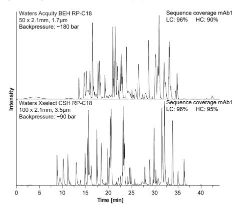
**Figure 2.** Comparison of two different RP-C18 columns in the mD-LC-MS set-up using mAb1, prior flow rate and temperature optimization. The Waters Acquity BEH RP-C18 column (particle size 1.7  $\mu$ m, 50 x 2.1 mm) (Top) and the Waters XSelect CSH RP-C18 column (particle size 3.5  $\mu$ m, 100 x 2.1 mm) (Bottom). A detailed overview of the identified peptides for both columns is shown in **Table S2.**
