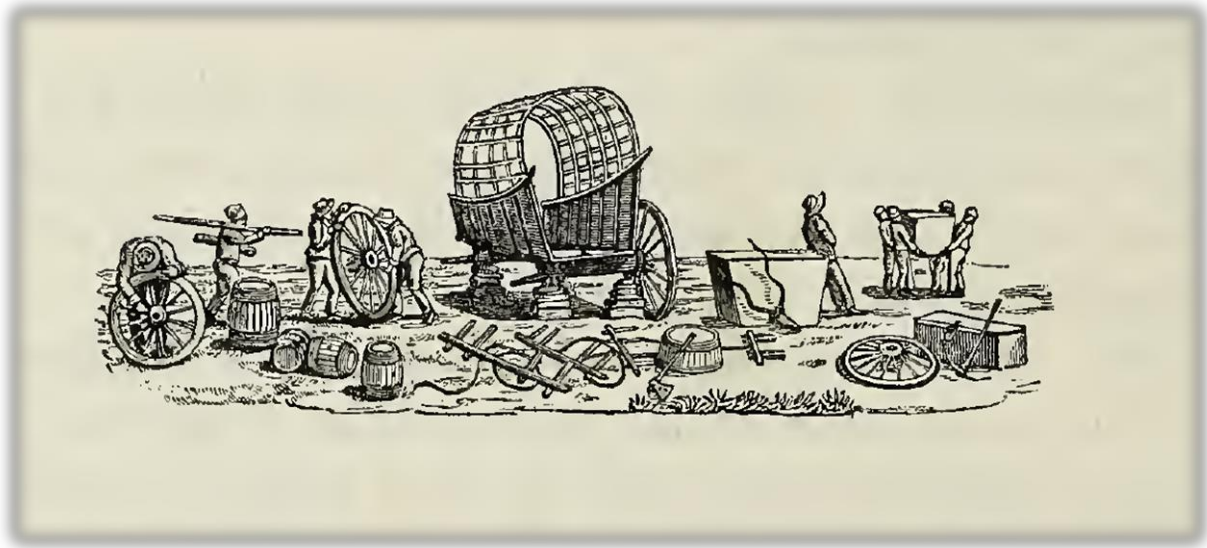
Image 2.3. William Burchell's depiction of a wagon being dismantled to change a wheel
