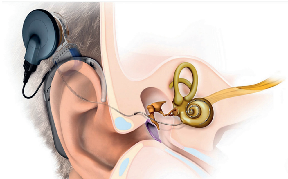
Figure 1: Illustration of a cochlear implant device (right ear) with the external and internal components. The external components include the microphone, speech processor and headpiece. The internal components consist of the internal receiver, internal wire and electrode array inside the cochlea. Image courtesy of Prof. Völter, head of Hearing competence centre Ruhr-University Bochum, Germany.
