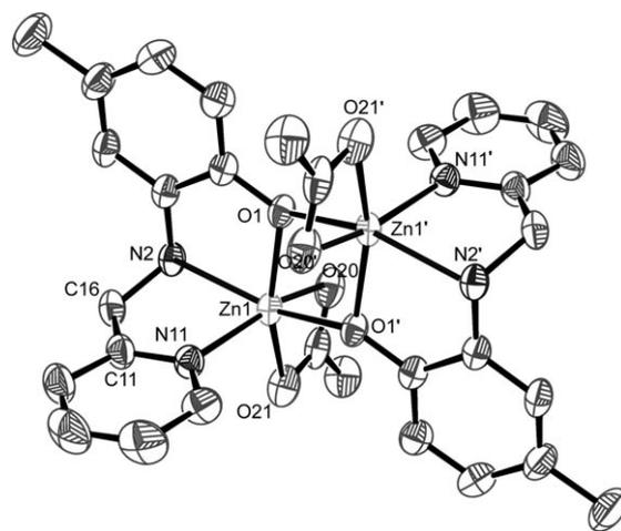
Figure 1. ORTEP perspective view of zinc(II) complex **2**. Hydrogen atoms and lattice solvent molecules have been omitted for clarity. Selected bond lengths [Å] and angles [°]: Zn1–O1 2.018(3), Zn1–O1' 2.063(2), Zn1–O20 2.315(3), Zn1–O21 2.109(3), Zn1–N2 2.211(3), Zn1–N11 2.090(3); O1–Zn1–N11 104.93(11), N11–Zn1–O21 98.45(12), O21–Zn1–O20 58.40(11), O20–Zn1–O1 98.02(11), N2–Zn1–O1' 156.73(11). Symmetry operation:  $1-x, -y, 1-z$ .
