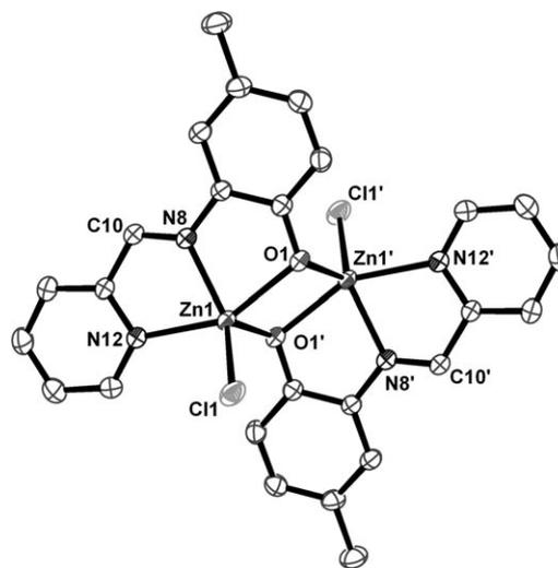
Figure 7. ORTEP perspective view of zinc(II) complex **5**. Hydrogen atoms have been omitted for clarity. Selected bond lengths [Å] and angles [°]: Zn1–O1' 1.9894(10), Zn1–O1 2.1770(10), Zn1–Cl1 2.2269(4), Zn1–N8 2.0691(12), Zn1–N12 2.2113(13); O1'–Zn1–Cl1 111.00(3), Cl1–Zn1–N8 131.02(4), N8–Zn1–O1' 117.55(5), N12–Zn1–O1 152.67(4). Symmetry operation':  $-x, -y, -z$ .
