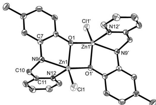
Figure 2. ORTEP perspective view of zinc(II) complex **3**. Hydrogen atoms and lattice solvent molecules have been omitted for clarity. Selected bond lengths [Å] and angles [°]: Zn1–O1 2.0192(10), Zn1–O1' 2.0838(10), Zn1–Cl1 2.2575(4), Zn1–N9 2.2088(13), Zn1–N12 2.0658(12); O1–Zn1–Cl1 134.53(3), Cl1–Zn1–N12 116.22(4), N12–Zn1–O1 107.95(5), N9–Zn1–O1' 155.39(5). Symmetry operation':  $1-x, 1-y, 1-z$ .
