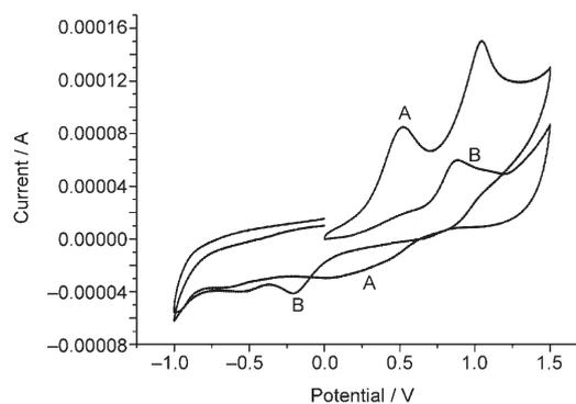
Figure 16. Cyclic voltammograms of 0.001 M complex **2** (A) and 0.001 M complex **1** (B) in DMF, at room temperature, versus Ag/Ag<sup>+</sup>.
