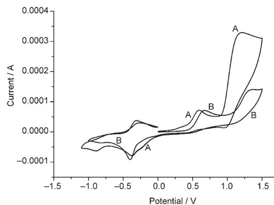
Figure 17. Cyclic voltammograms of 0.001 M complex **3** (A) and 0.001 M complex **5** (B) in DMF, at room temperature, versus Ag/Ag<sup>+</sup>.
