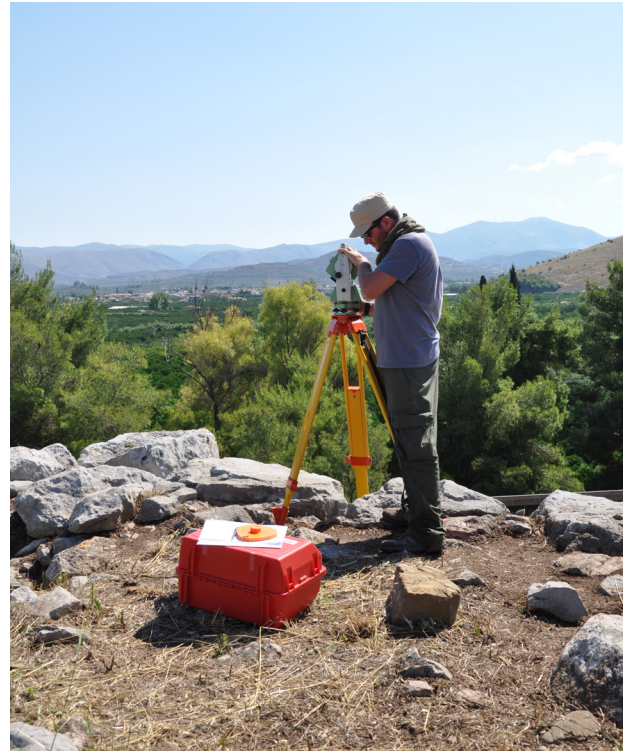
Figure 3. Employing the reflectorless total station to measure geo-referenced photomarkers on site during the Tiryns fieldschool with colleague Alexis Gorgues in 2015 (figure A. Brysbaert).
