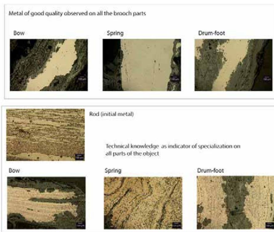
Figure 7: Photomicrographs of different parts of the brooches studied, showing the quality of the metal used up in the figure, and the nature of the metal and the work of the smith for each part down in the figure. (Pictures and drawings: A. Filippini).
