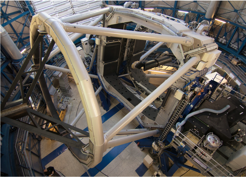
Figure 1.1: Unit Telescope 3 of the Very Large Telescope with SPHERE installed on the Nasmyth platform (bottom right). Image credit: J. H. Girard / ESO.
