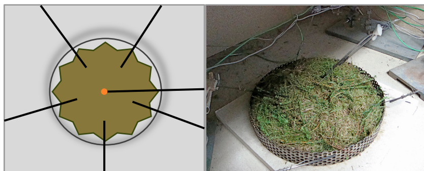
Figure 1. Schematic design and true image of the fire experiment fuel bed; the schematic design includes fuel, thermocouples, and the position of ignition.
