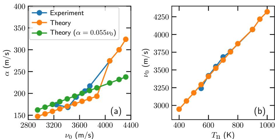
FIGURE 8.2: Width parameter  $\alpha$  as a function of the stream velocity  $\nu_0$  (a) and the stream velocity  $\nu_0$  as a function of the nozzle temperature  $T_n$  (b). Experimental parameters[9] and parameters used in this work are indicated in blue and orange, respectively. Theoretical parameters where  $\alpha = 0.055\nu_0$  are indicated in green.
