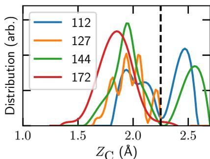
FIGURE 8.6: Distributions of the height of the carbon atom when a CH-bond dissociates (i.e.,  $r = r^\ddagger$ ) for  $\nu_1 = 2$  at various incidence energies (numbers are in kJ/mol). The TS geometry value for  $Z_C$  is indicated by the dashed line.
