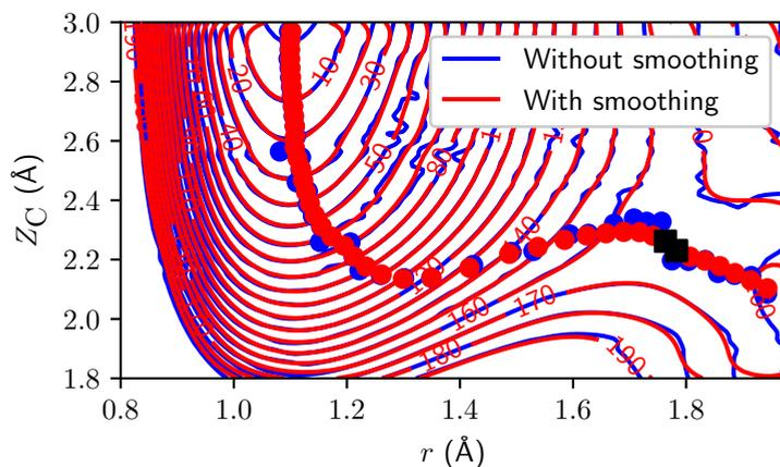
FIGURE 8.B.1: Elbow plot of methane on Cu(111) obtained with the HD-NNP with (red) and without (blue) smoothing, where  $Z_C$  and  $r$  (distance between the carbon atom and surface, and the length of the dissociating CH bond, respectively) are variable. Contour lines are drawn at intervals of 10 kJ/mol between 0 and 200 kJ/mol. The circles indicate the MEP and the black squares indicate the highest point along the MEPs.
