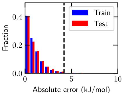
FIGURE 8.4: Distribution of absolute total energy errors (kJ/mol) of the HD-NNP compared to the DFT total energy. Blue indicates the training set, whereas red indicates the test set. The dashed line indicates chemical accuracy, i.e., 4.2 kJ/mol.
