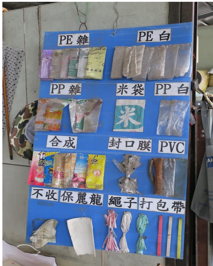
Figure 4.1 Reference sample board of Tzu-chi plastic packaging material classification (photo by the author, 2016)
